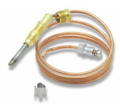
Robertshaw® thermocouples are the industry leader for gas heating and appliances. Their primary function is to ensure a standing pilot light is operative so that on a call for heat, the main burner gas will be properly ignited. Thermocouples are placed in gas applications to detect existence of a flame for safety purposes by shutting off the potential gas flow to a burner.
